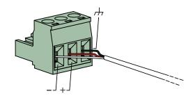
For unbalanced signal input connections
