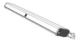
To prevent the soundbar from falling down, the security screw on top of the fixation hooks shall be tightened.
