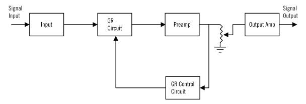
Figure 1 - Block Diagram of the 1176
