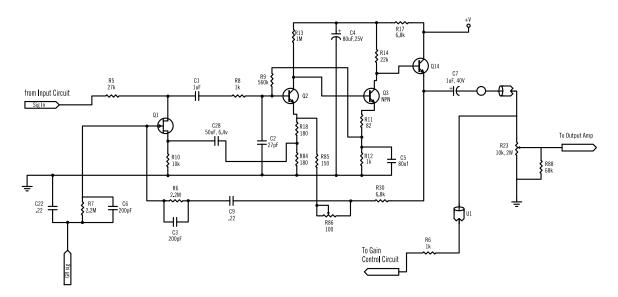
Figure 3 - Gain Reduction Stage
