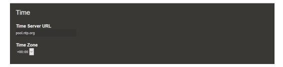
In case your system is restricted from access to internet, an internal time server on your LAN network should get assigned offering synchronization to the system. The IP address of the internal time server should be entered in the text field instead of the standard value 'pool.ntp.org'
