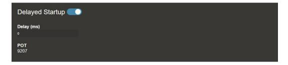
The delayed startup can be activated through enabling the indicated button, and the delay time (the delay between each two relays triggering) can be configured analogue (through a potentiometer located on the ARU20x PCB) or digitally through entering a milliseconds value inside the corresponding text field.
