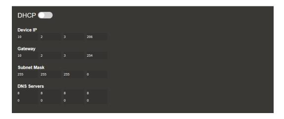
The DCHP function is standard switched off and can be turned one by clicking and enabling the corresponding indicator.
