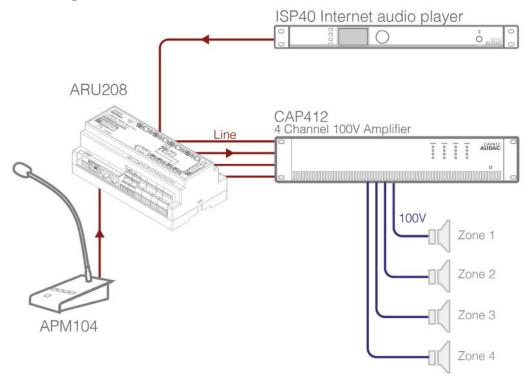
The above diagram shows an example of a simple and basic setup with an APM1xx paging console in an analogue paging setup, combined with an ARU20x relay unit. Besides the APM1xx paging console, a background music source (ISP40 in this typical setup) is connected.
