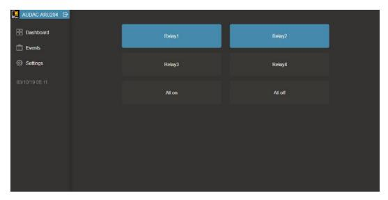
The text inside the relay knob is default shown as 'Relayx' where x represents the number of the corresponding relay (1 up to 4 for ARU204 or 1 up to 8 for ARU208). This text can be adjusted according to customers preferences, allowing to create a more clear and intuitive interface for the user.
