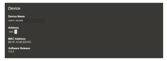
The device address is an unique address which shall be used when multiple units are daisy—chained with each other and addressed through a single IP address. Each device in the chain should have an unique device address which is selectable between 'S001' and 'S099'.
