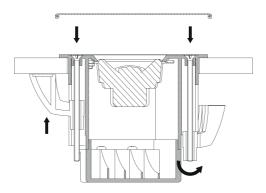
6) After the screws are tightened and the speaker is level with the surface, the front grill can be assembled to the loudspeaker.
