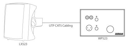
In the most common applications the LX523 active speaker system will be used in combination with the WP523 wall panel. This wall panel contains an unbalanced line input (RCA) and balanced microphone input (with phantom power). Both input channels have local mixing which can be controlled through the push-lock potentiometers, and the master volume can be controlled by means of the big dial.
