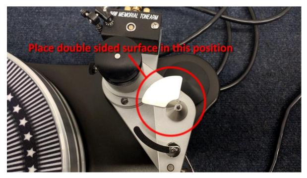
Use the provided Allen wrench to attach the Pivot Clamp to your tonearm and the same Allen Wrench to adjust the height of the Pivot Point. This is how you will be able to adjust the Azimuth of your tonearm if you choose not to use the drop-counter weight or the side Azimuth weights (Note: some VPI model tonearms do not have adjustable side weights).
