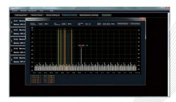
Scanning: Obtain scan data through Relacart wireless receivers and compatible scanners, provide detailed graphic displays, and detect potential RF problems in time to avoid adverse effects on RF signals.
