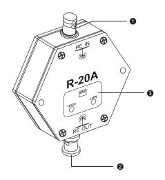
①The input connector of the antenna (BNC connector) and directly connect the BNC connector to R-20U antenna. ②Using high quality low loss coaxial cable to connect the output connector (BNC connector) of R-20A to the input of Relacart UHF receiver or R-14D Antenna Divider. And this connector also output power to the R-20A UHF Wide-band Directional Antenna.
